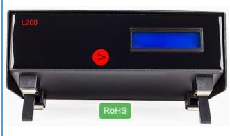
The Labfacility L200 TC thermocouple thermometers (Temperature Logger) can be used in conjunction with a PC to provide accurate, versatile 8 channel thermocouple temperature measurement, scanning and logging of measured values. It can also be used as a stand alone indicator/logger and incorporates a digital display of measured temperature.
