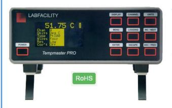
The Tempmaster PRO provides precise Platinum Resistance Thermometer temperature measurement and logging for exacting applications in both laboratory and site locations. It is an exceptionally accurate and stable digital thermometer particularly suitable for use with thermal calibration baths as a reference standard.
