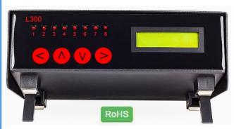
The Labfacility L300 Pt100 temperature alarm / on-off controller can be used in conjunction with a PC to provide accurate monitoring and alarm or on-off control of up to 8- zones simultaneously. It can also be used as a stand-alone instrument without the need for a PC.
